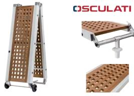
Made of anodized aluminium, foldable in two pieces, fitted with genuine Siam **real teak grating**; supplied with two **stainless steel** stanchions, rubber wheels, **stainless steel** pivot pin and flush-mount bushing. Fastening bushing  $\emptyset$  25mm.
