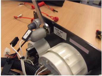
Tighten the nut on the backside of the panel
