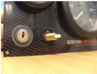
Remove the cap and washer from the new switch and put it through the hole
