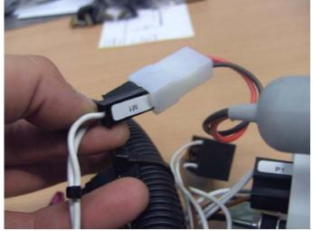
Connect the kill switch to the connectors marked M1 and M2. The polarity is not important.
