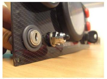
Put the washer and the cap back on and tighten the cap as much as possible by hand
