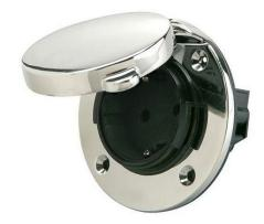
Schuko outlet socket for exterior application. The Schuko socket is a high quality in-wall outlet designed for outdoor use. The high-gloss polished stainless steel cap and flange warranty a long lasting stylish look. When the bayonet cap is closed the outlet is protected against water ingress (IP56).
