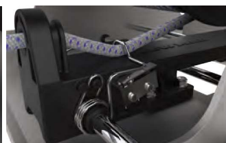
The composite rode feeder arm includes a sprung load-detecting device. This prevents the unit from paying-out when the line is slack.
