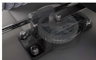
Manufactured in robust acetal, a compact worm and wheel gear system powers the rode feeder arm, thereby neatly laying the rode on the drum.
