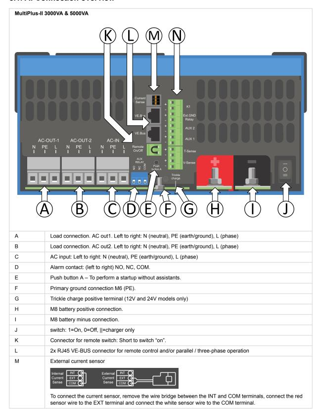
Ν Terminal for: top to bottom: 12V 100mA 2. Programmable contact K1 open collector 70V 100mA External ground relay + 3. External ground relay -4. 5. Aux input 1 + 6. Aux input 1 -7. Aux input 2 + Aux input 2 -8. Temperature sense + 9. 10. Temperature sense -11. Battery voltage sense + 12. Battery voltage sense -
