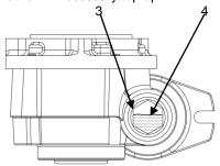
Clean the Windlass with a cloth damp with Kerosene (paraffin). Spray preferably with CRC3097 "Long Life" or alternatively, CRC6-66 or WD40 (or alternative). Polish off with a clean nonfluffy cloth.
