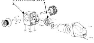
Check level of oil in gearbox using the sight glass
